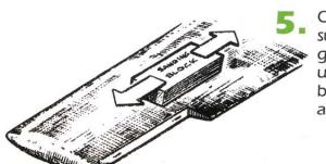
Once cured, sand surface with 220 grit sandpaper using sanding block. Then prime and paint.
