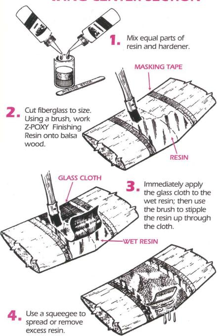
S Allow resin to cure; then use a sanding block to level the
