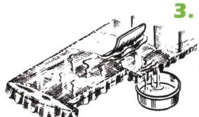
Using a spreader, "squeegee" excess resin into container, leaving a thin surface of fiberglass and resin. Allow to cure for 3 hours.
