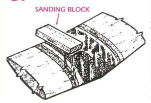
major bumps and lumps. Flow on a second coat of resin which should be allowed to cure before sanding to a fine finish. Remove masking tape last so that balsa wood wing skin is always protected from the sanding block.
